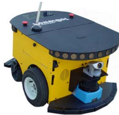
Figure 7. PowerBot™ carries over 100 kg of payload.
