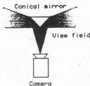
Figure 2 - The omnidirectional perception device.
